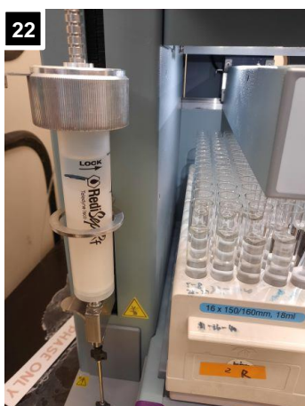
22: Crude product is purified by ion exchange chromatography on DEAE-Sephadex.
